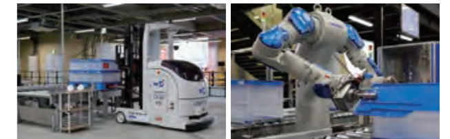
Unmanned forklift system
