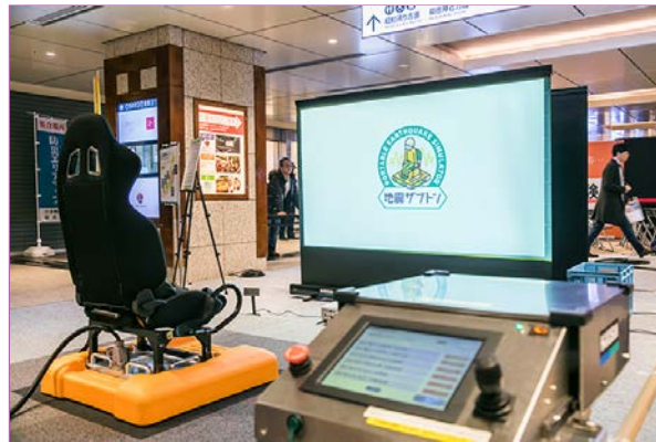
► This "earthquake chair" simulates the effects of a temblor based on data from major quakes
