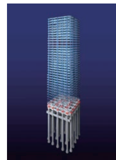
Seismic isolation structure using deep piles
